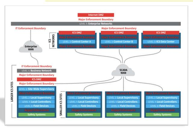
Zones and zone separation. The architectural structure described in the model above defines a separation of zones within the SCADA architecture. This separation is based on different tasks or categories of the systems within the architecture. Systems belonging to a certain category, or "SCADA level", are only intended to communicate with "neighboring" SCADA levels.
